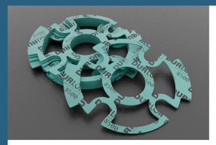
Durlon® RCA® sealing system combined with Durlon® PTFE styles can replace standard full gaskets in FRP, PVC and other non-metallic and metallic pipe flanges where a low stress gasket is required. The RCA® configuration can be cut from standard PTFE & CNA sheets resulting in a cost savings versus other low stress gaskets.
