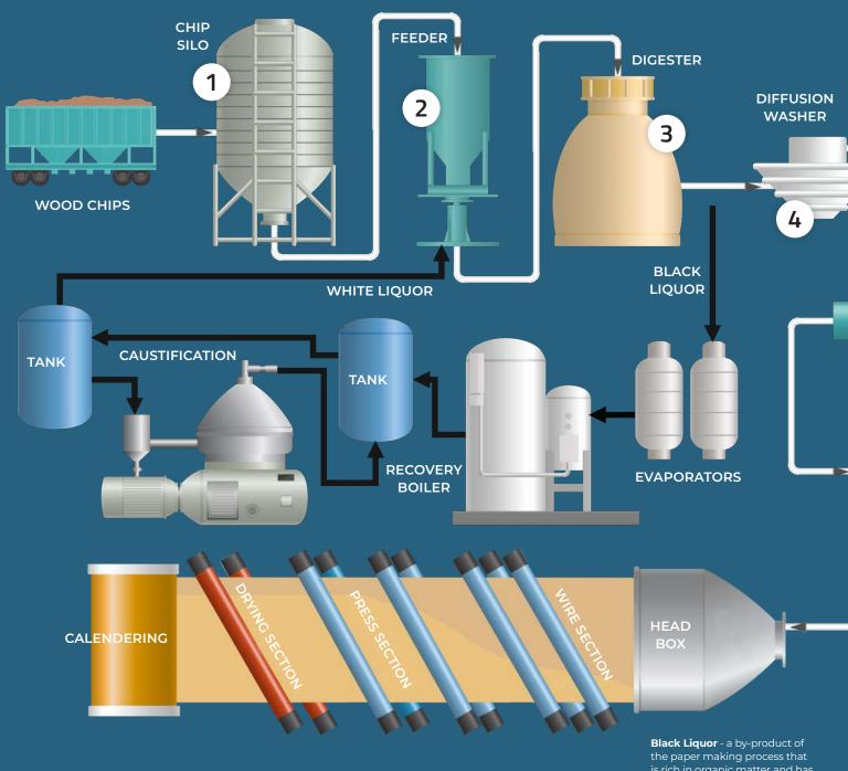
NOTE: This is a graphical representation of a pulp and paper production process, showing the primary process flow path. It does not show the minor details of the process, rather it focuses on the equipment used, and other instruments that are present. It helps to illustrate how the major components of this type of process plant interacts with each other to bring about the desired effect.
