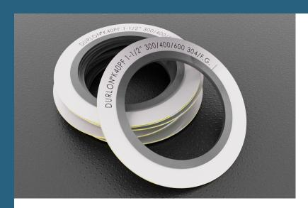
Durlon® Kammprofile gaskets have a solid metal core with concentrically serrated grooves machined into the top and bottom faces. The metal core is typically stainless steel, but it can be supplied in various metallurgies as per the customer's request.
