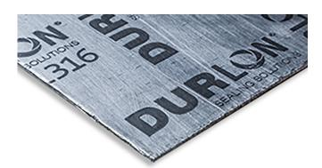
**FGL316:** Standard industrial grade sheet laminated with an adhesive bond on both sides of a 0.002" thick 316 stainless steel foil core. This product is used where high performance and handling are important.
