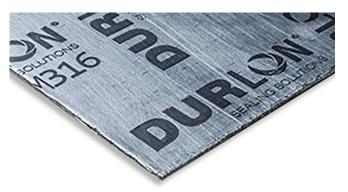
**FGM316:** Inhibited grade sheet laminated with multiple layers of 0.004" thick 316 stainless steel foil core. This product is used in applications with high mechanical stress or pressure, above average burst resistance, exceptional rigidity, and suitable to cut gaskets with narrow strips.
