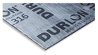
**FGL316:** Standard industrial grade sheet laminated with an adhesive bond on both sides of a 0.002" thick 316 stainless steel foil core. This product is used where high performance and handling are important.
