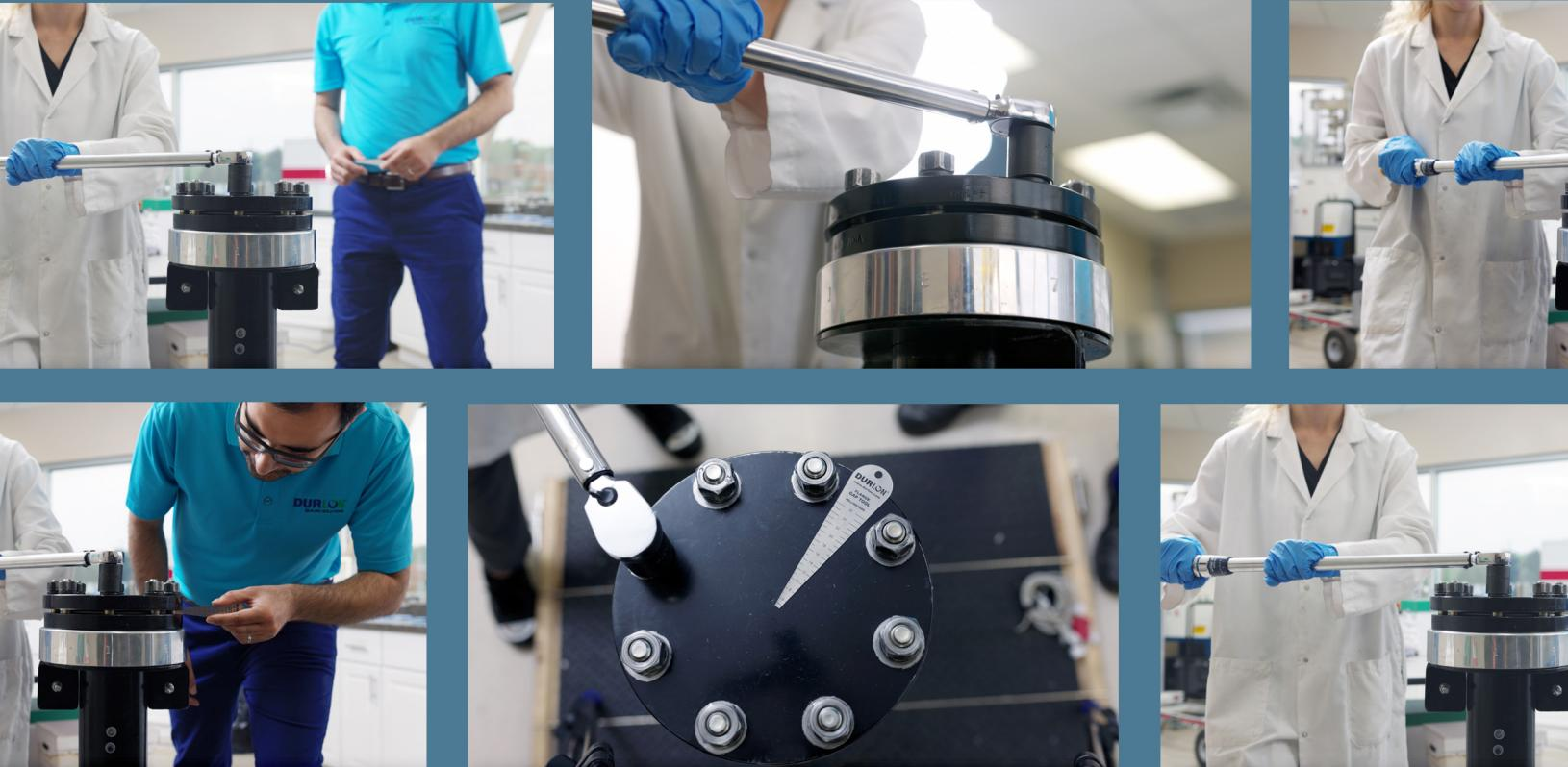
Proper torque values are essential not only for achieving an effective seal but also for ensuring the longevity and reliability of the gasket and the overall system. Insufficient torque can result in inadequate compression, leading to gaps and uneven pressure distribution on the gasket. This can cause leaks and compromise the system's performance. On the other hand, excessive torque may deform the gasket, leading to its premature failure or damage to the mating surfaces.
