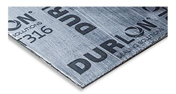
**FGT316:** Standard industrial grade sheet mechanically bonded on both sides of a 0.004" thick 316 stainless steel tang core. This product is used where stresses and pressures are high and improved handling is important.
