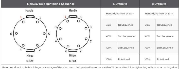
Retorque after 4 to 24 hrs. A large percentage of the short-term bolt preload loss occurs within 24 hours after initial tightening with most occurring after 4 to 5 hours. This Round recovers this loss. Failure To Pre-Tighten The Nuts Result In Flanges That Are Not Parallel, And Could Result In Possible Leakage.
