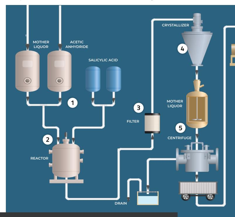
NOTE: This is a graphical representation of an aspirin production process, showing the primary process flow path. It does not show the minor details of the process, rather it focuses on the equipment used, and other instruments that are present. It helps to illustrate how the major components of this type of process plant interacts with each other to bring about the desired effect.
