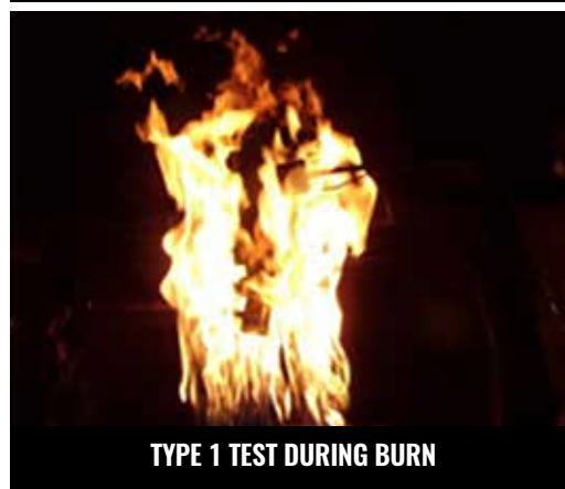
Figure 1: API 6FB Type 1 (Onshore) Test Setup Prior to Burn (Top) and Test During Burn (Bottom).
