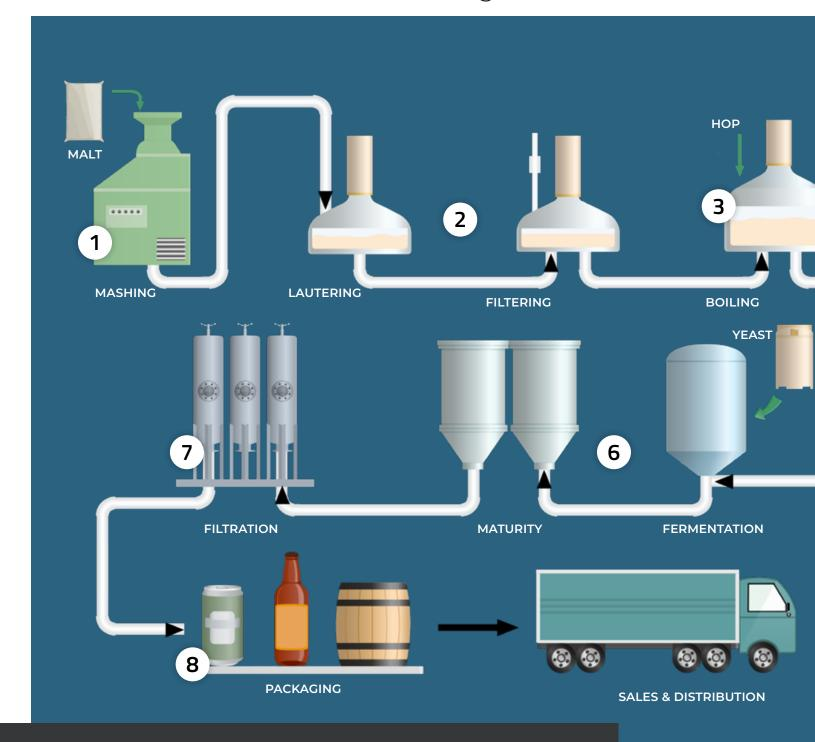
NOTE: This is a graphical representation of a beer production process, showing the primary process flow path. It does not show the minor details of the process, rather it focuses on the equipment used, and other instruments that are present. It helps to illustrate how the major components of this type of process plant interacts with each other to bring about the desired effect.
