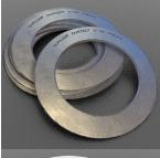
**Durlon® Durtec®** gaskets are made with a specially engineered corrugated metal core that is bonded on both sides with soft covering layers, typically flexible graphite. The core is produced by patented technology that allows the finished gasket to have the best possible mechanical support function. Corrugations in the core are virtually un-crushable unlike conventional corrugated metal core gaskets.
