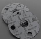
**Durlon® 8900** is a premium grade material for service conditions to 496°C (925°F) and continuous operating temperatures of -73°C to 400°C (-100°F to 752°F). Suitable for saturated and superheated steam, oil, dilute acids and alkalis, hydrocarbons, and solvents.
