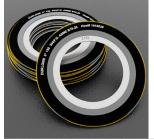
**Durlon® Spiral Wound (SWG DRI FG)** Gaskets are made with an alternating combination of a preformed engineered metal strip and a more compressible filler material which creates an excellent seal when compressed. The engineered shape of the metal strip acts as a spring under load, resulting in a very resilient seal under varying conditions.
