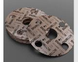
**Durlon® HT1000®** consists of phlogopite mica paper impregnated with an inorganic binder at less than half the binder amount found in vermiculite-phyllosilicate filled products. This lower binder content allows for superior weight retention, less than 4% weight loss at 800°C (1,472°F), and results in ultimate extreme temperature sealing performance up to 1,000°C (1,800°F).
