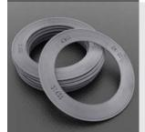
**Durlon® CFG** is a corrugated, flexible graphite gasket material designed for severe service conditions. The proprietary design of the corrugations gives CFG superior sealing and recovery characteristics for tough conditions in the refining, chemical, petrochemical and pulp and paper industries. Durlon® CFG is suitable for service in steam, oil, water, mild alkalis, mild acids, hydrocarbons and solvents.
