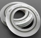
**Durlon® Spiral Wound (SWG DRI ETG)** Gaskets are made with an alternating combination of a preformed engineered metal strip and a more compressible filler material which creates an excellent seal when compressed. The engineered shape of the metal strip acts as a spring under load, resulting in a very resilient seal under varying conditions.
