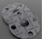
**Durlon® 8900** is a premium grade material for service conditions to 496°C (925°F) and continuous operating temperatures of -73°C to 400°C (-100°F to 752°F). Suitable for saturated and superheated steam, oil, dilute acids and alkalis, hydrocarbons, and solvents.
