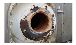
Many of the aging plants we service are run beyond their expected life cycle and over time, metal piping, including flanges can corrode and become worn due to various reasons, making flange conditions a very important part of creating an effective gasket seal.
