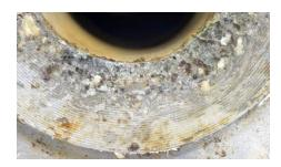
Shutdowns cost industry millions. And a significant impact on operating costs can be due to corrosion, or damaged flange faces. When corrosive media meets the sealing surfaces of facing flanges a leak WILL occur. So, flange maintenance is an important step to help prevent leakage.
