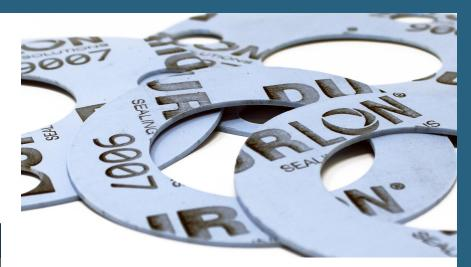
Durlon® 9007 is formulated with a homogenous blend consisting only of pre-shaped inorganic fillers, pure PTFE resins, and pigment. It is suitable for use in steel flanges and does not exhibit the cold flow problems associated with virgin PTFE or the hardness problems of silica-filled PTFE. Unlike generic glass fibre filled PTFE, the shapes of the fillers used in Durlon® 9007 do not allow wicking of media through the gasket which can lead to corrosion on flange surfaces.
