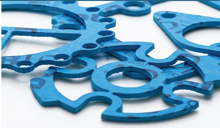
Durlon® 8700 is a high performance gasket material for use in processes requiring a neoprene (CR) bonded sheet and has excellent hand and die cutting characteristics. This product has excellent resistance to ozone, oils, non-aromatic solvents and many refrigerants.
