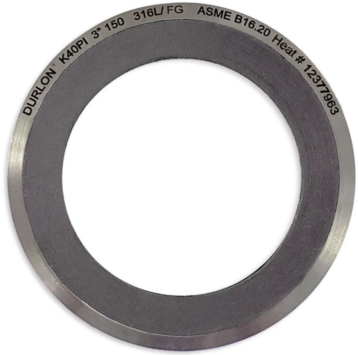
Durlon® Kammprofile gaskets have a solid metal core with concentrically serrated grooves machined into the top and bottom faces. The metal core is typically stainless steel, but it can be supplied in various metallurgies as per the customer's request.
