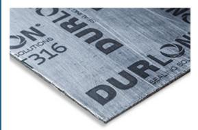
FGT316: Standard industrial grade sheet mechanically bonded on both sides of a 0.004" thick 316 stainless steel tang core. This product is used where stresses and pressures are high and improved handling is important.
