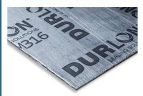
**FGM316:** Inhibited grade sheet laminated with multiple layers of 0.004" thick 316 stainless steel foil core. This product is used in applications with high mechanical stress or pressure, above average burst resistance, exceptional rigidity, and suitable to cut gaskets with narrow strips.
