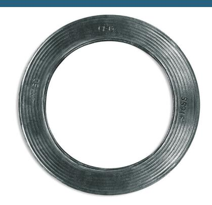
Durlon® CFG is a corrugated flexible graphite gasket material designed for severe service conditions. The proprietary design of the corrugations gives Durlon® CFG superior sealing and recovery characteristics for tough conditions in the refining, chemical, petrochemical and pulp & paper industries. Durlon® CFG is suitable for service in steal, oil, mild alkalis, mild acids, hydrocarbons and solvents.
