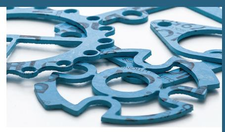
Durlon® 7950 is an economy grade general service gasket sheet material made with NBR (Nitrile Butadiene Rubber) binder for mild service in piping and equipment with applications in steam, hydrocarbons and refrigerants and an alternative when temperature and pressure conditions are below 500°F (260°C) and 1,200 psig (See PxT chart below for validation).
