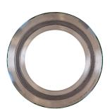
**Durlon® Spiral Wound (SWG DRI ETG)** Gaskets are made with an alternating combination of a preformed engineered metal strip and a more compressible filler material which creates an excellent seal when compressed. The engineered shape of the metal strip acts as a spring under load, resulting in a very resilient seal under varying conditions.
