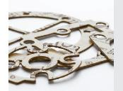
**Durlon® HT1000®** consists of phlogopite mica paper impregnated with an inorganic binder at less than half the binder amount found in vermiculite-phyllosilicate filled products. This lower binder content allows for superior weight retention, less than 4% weight loss at 800°C (1,472°F), and results in ultimate extreme temperature sealing performance up to 1,000°C (1,800°F).
