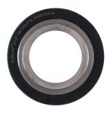
**Durlon® Spiral Wound (SWG DRI FG)** Gaskets are made with an alternating combination of a preformed engineered metal strip and a more compressible filler material which creates an excellent seal when compressed. The engineered shape of the metal strip acts as a spring under load, resulting in a very resilient seal under varying conditions.
