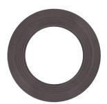
**Durlon® Durtec®** with Durcore® gaskets are made with a specially engineered corrugated metal core that is bonded on both sides with soft covering layers, typically flexible graphite. The core is produced by patented technology that allows the finished gasket to have the best possible mechanical support function. Corrugations in the Durtec® core are virtually un-crushable unlike conventional corrugated metal core gaskets.
