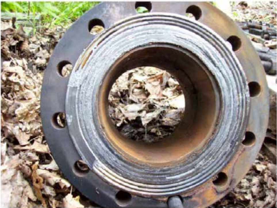
Gasket After Test - End of 30 minute Burn and 10 minute Cooldown
