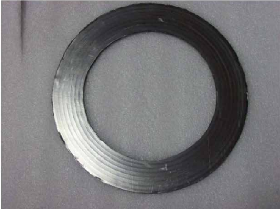
Sample of Gasket Before Test - 6 inch Class 300 Durlon® Durtec® Gasket
