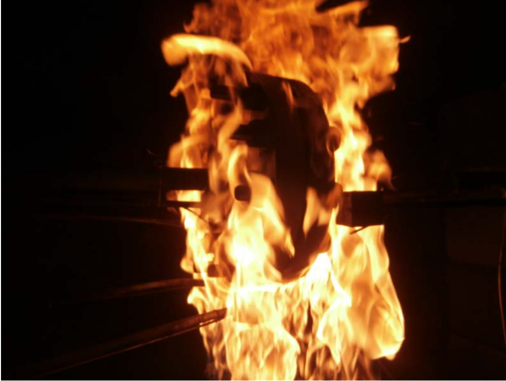
Test Gasket During Burn
