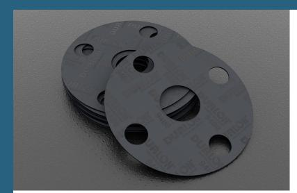
Durlon<sup>®</sup> 9400 is a high performance filled PTFE gasket material designed for use in piping and equipment, chemical, and other general industrial applications where resistance to highly aggressive chemicals (including hydrofluoric acid) is required. Durlon<sup>®</sup> 9400 can also be used as the gasket of choice for anhydrous hydrogen fluoride (AHF) in railroad tank cars and a good alternative for use in plants where barium sulfate filled PTFE may not be suitable.
