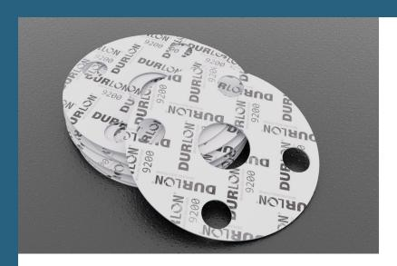
Durlon® 9200 is a filled PTFE gasket material used where resistance to highly aggressive chemicals is required. Barium sulfate fillers are homogeneously blended with pure PTFE resins to give Durlon® 9200 its physical and mechanical properties.
