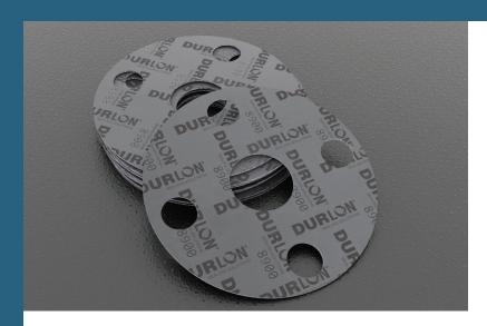
A premium grade material for service conditions to 496°C (925°F) and continuous operating temperatures of -40°C to 400°C (-40°F to 752°F). Durlon® 8900 is ideal for saturated and superheated steam, oil, dilute acids and alkalis, hydrocarbons and solvents.
