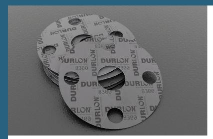
Durlon<sup>®</sup> 8300 is a premium grade compressed sheet gasket material that is excellent in steam and hydrocarbon services for the refining, petrochemical, and power generation industries. This gasket material is designed to handle the extreme pressure and temperature applications that include oil, water, mild alkalis, mild acids and solvents.
