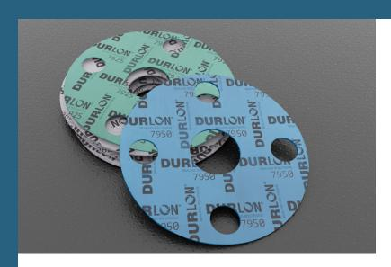
Durlon® 7900/7925/7950 are an economy grade general service gasket sheet material made with NBR (Nitrile Butadiene Rubber) binder for mild service in piping and equipment with applications in steam, hydrocarbons and refrigerants and an alternative when temperature and pressure conditions are below 500°F (260°C) and 1,200 psig (See PxT chart below for validation).
